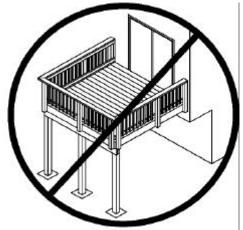
FIGURE 10: NO ATTACHMENT TO HOUSE OVERHANG
